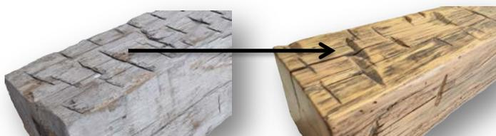
**2. Sand:** Using either a belt sander or sanding by hand, Trestlewood uses progressively finer sandpaper (100, 150 and then 220 grit) to smooth out and/or remove any undesired texture or features.
